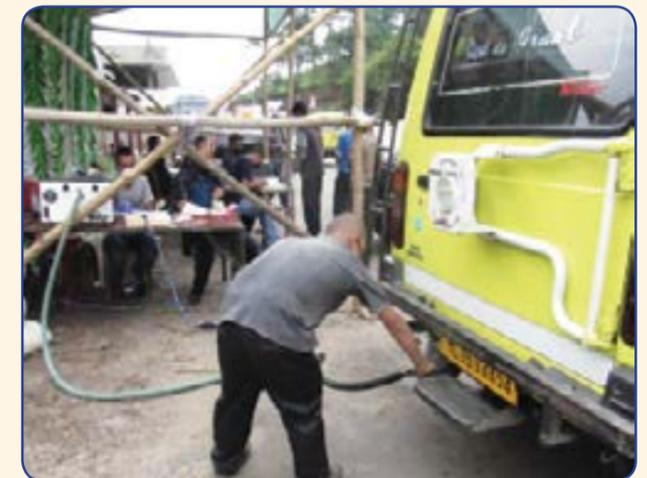
Emission test of Diesel driven vehicle in progress
