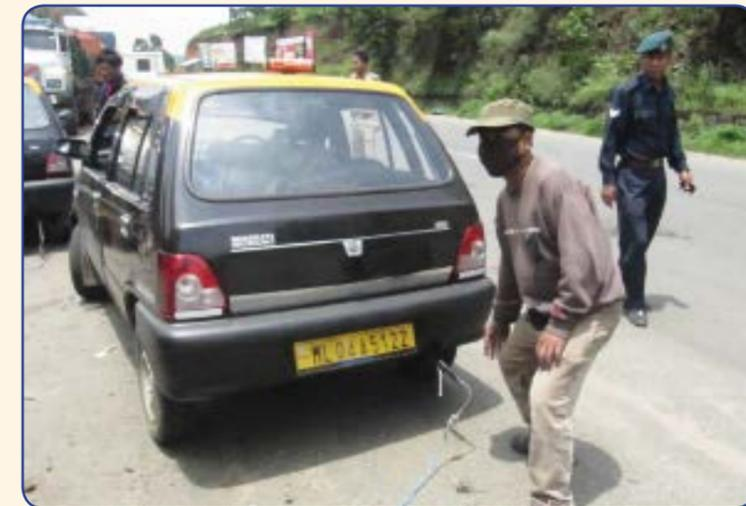
Emission test of Petrol driven vehicle in progress
