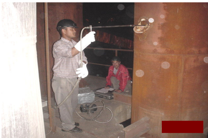
Monitoring of emission from the chimney of Industry to verify compliance with the prescribed Stack-Emission Standards.
